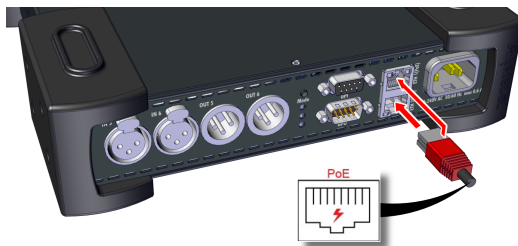
figure 13: powering via PoE
