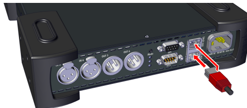
figure 11: connecting AES67 network
