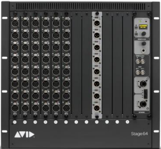
Stage 64 I/O Rack
