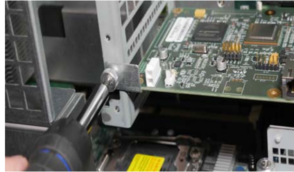
Figure 22. Securing the card to the back bracket
