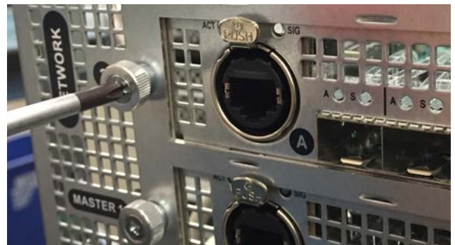
Figure 5. Loosening the exterior thumbscrew
