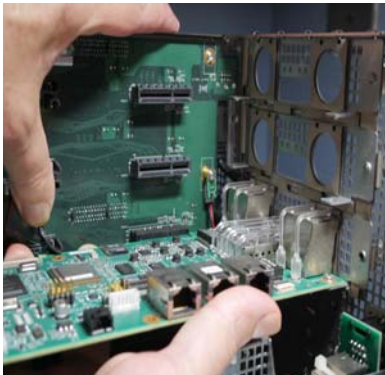
Figure 7. Lifting the tab using a thumb and disconnecting the AVB-192 card from its PCIe slot
