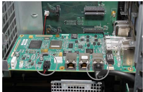
Figure 4. AVB-192 cables to disconnect (Master AVB-192 shown)
