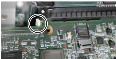
Figure 21. Retaining clip closed, when card is fully seated
