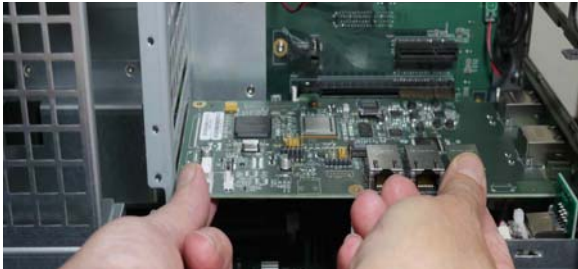
Figure 20. Guiding the WSG-HD Card into position
