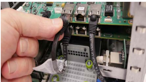
Figure 36. Ethernet connection from WSG-HD to Master AVB-192 (E6L-192 or E6L-144 only)
