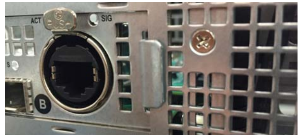
Figure 38. Proper position of the Network card faceplate tab
