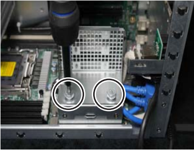
Figure 15. Removing the original Option Card bracket
