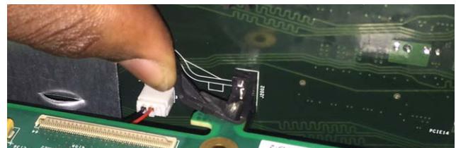
Figure 28. Lifting the tab on the retaining clip
