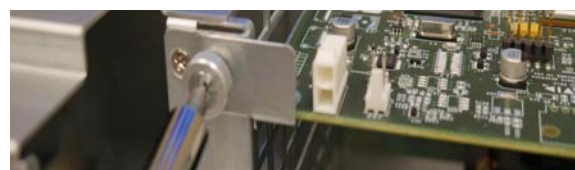
Figure 29. Securing the card to the back bracket
