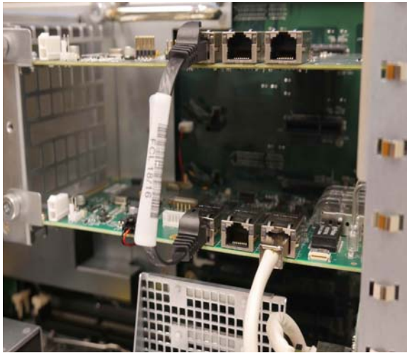
Figure 30. Ethernet connection from WSG-HD to Master AVB-192 (E6L-112 only)
