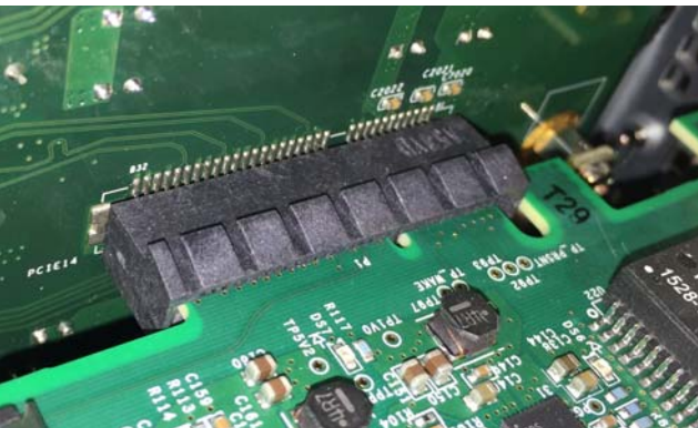
Figure 41. The Network card PCIe connector properly seated in the PCIe slot
