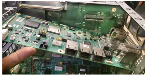
Figure 37. Placing the card into position inside the engine
