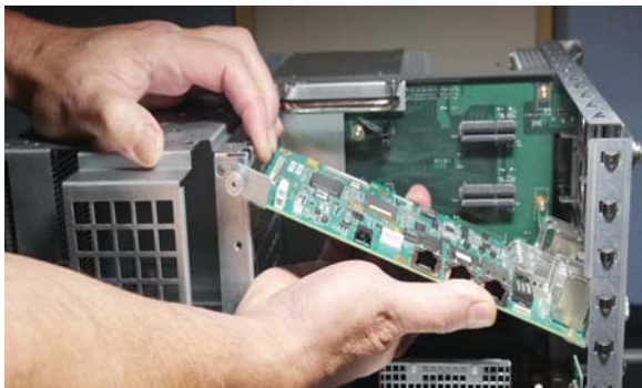
Figure 8. Removing an AVB-192 card
