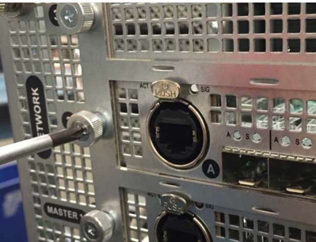
Figure 42. Tightening the exterior thumbscrew
