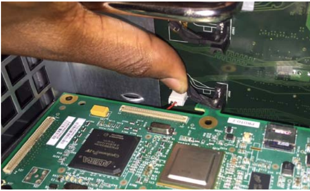
Figure 40. Lifting the tab on the retaining clip
