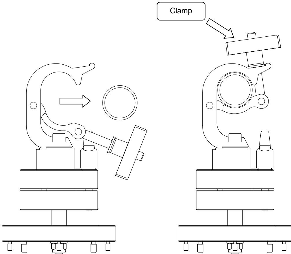
The device is operated by the locking lever, clamping is achieved by moving the lever to the left and releasing by moving to the right. If more or less clamping is required, lifting the lever will disengage it allowing it to be swivelled to the ideal clamping position. On releasing the lever it will automatically re-engage.
