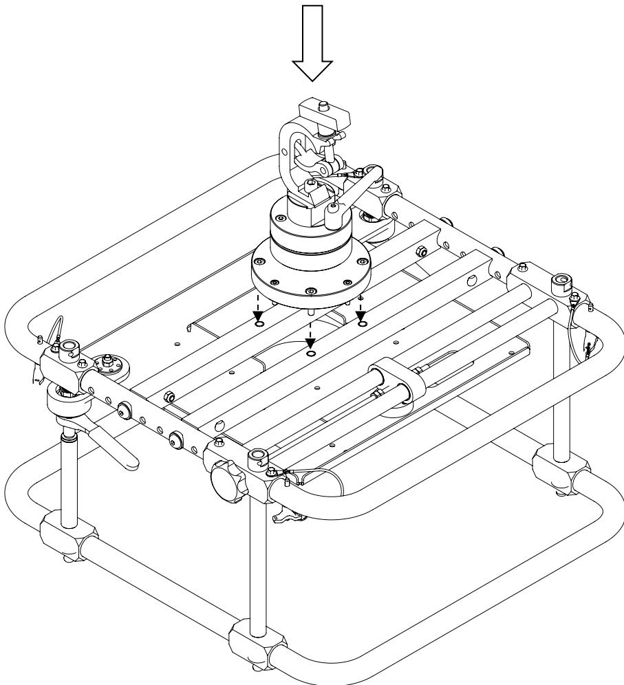
Loosen the clamp nut on the Atom Grip and lift onto the mounting truss (2 people may be required), once correctly located, tighten the clamp nut using hand pressure only.
