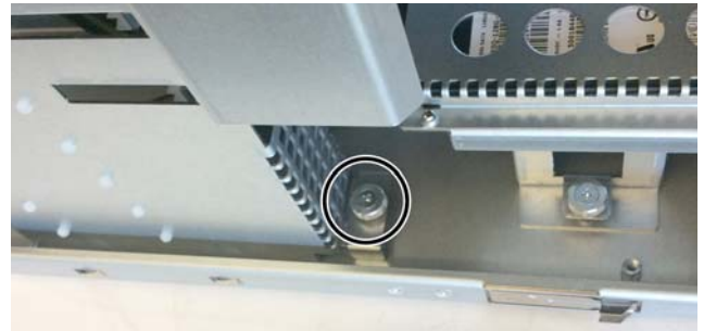
Figure 5. E6L card bracket thumbscrew
