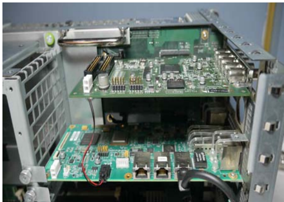
Figure 20. MADI-192 card properly seated in the PCIe slot
