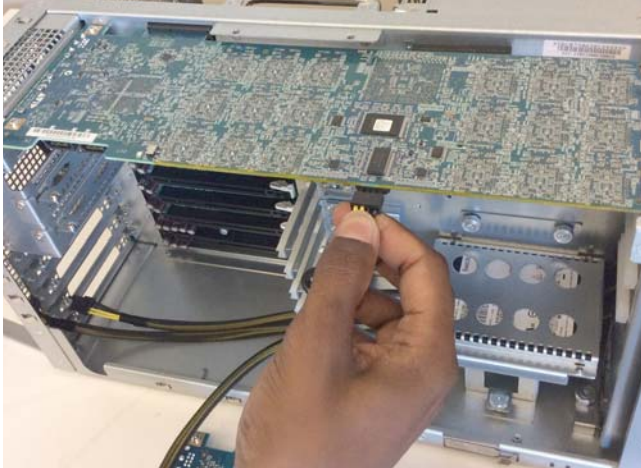
Figure 8. Disconnecting the power cable of an HDX card
