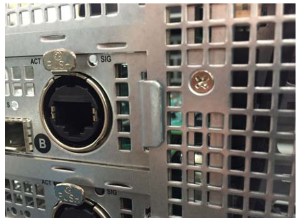
Proper position of the Network card faceplate tab
