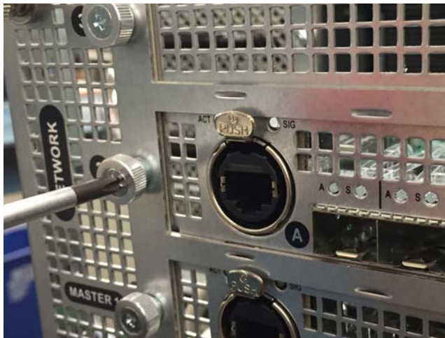
Tightening the exterior thumbscrew
