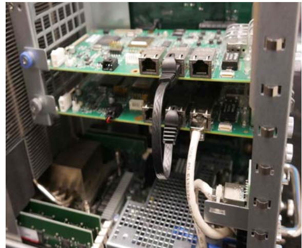
Ethernet cable connected between cards
