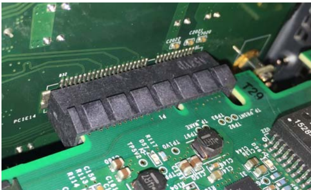
The Network card PCIe connector properly seated in the PCIe slot
