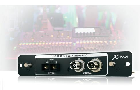
The X32's expansion slot provides flexible and expandable connectivity for many different applications. The X-MADI Expansion Card can easily be installed in place of the X-USB card that is included with the X32. The 32-channel interface brings even more I/O options to the X32 by instantly enabling it for MADI networking. The MADI or AES10 protocol is quickly becoming an industry standard in many broadcast applications.
