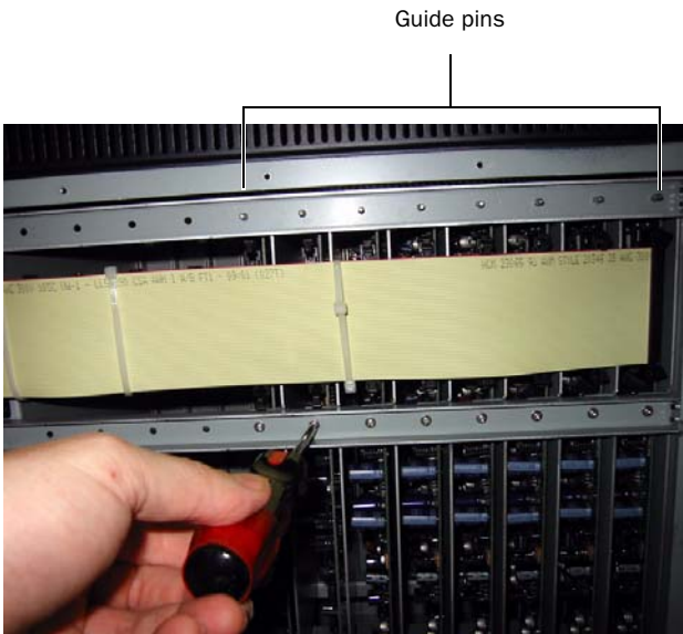
Securing a Stage Rack option card to the Stage Rack chassis
