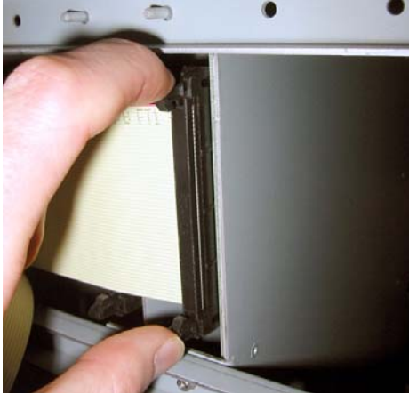
Connecting a Stage Rack option card to the Stage Rack ribbon cable
