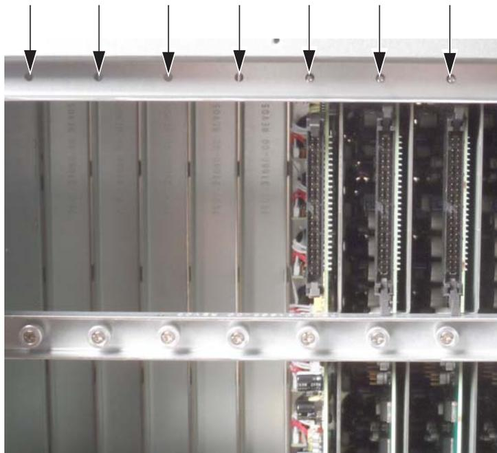
Figure 7. Guide pins and guide holes inside the Stage 64
