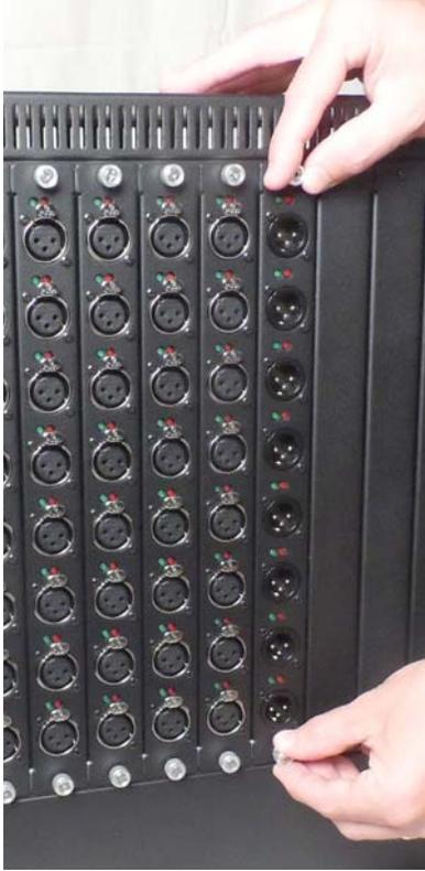
Figure 8. Tightening the front captive thumbscrews (Stage 64 shown)
