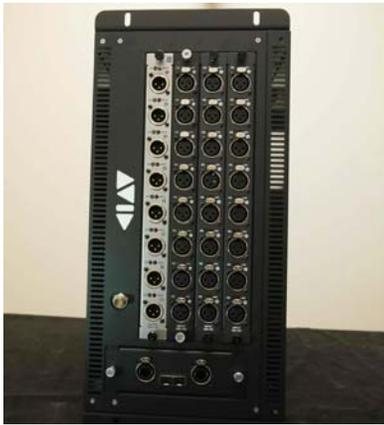
Figure 3. Stage 32 positioned for IO card installation
