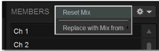
Removing all input assignments from a bus
