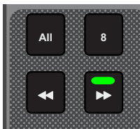
Fader Banking Navigation switches
