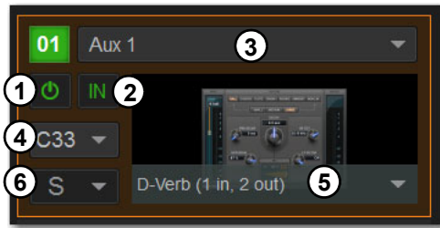
A rack slot and its controls, with an assigned plug-in shown
