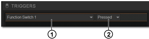
Properties for a switch trigger
