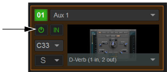
Rack slot power switch
