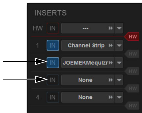
An engaged plug-in (top) and a disengaged plug-in (bottom)
