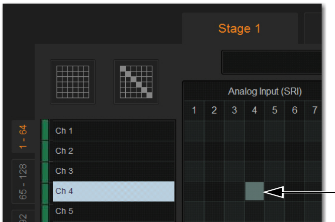
A lit grid square showing a hardware input source patched to an input channel
