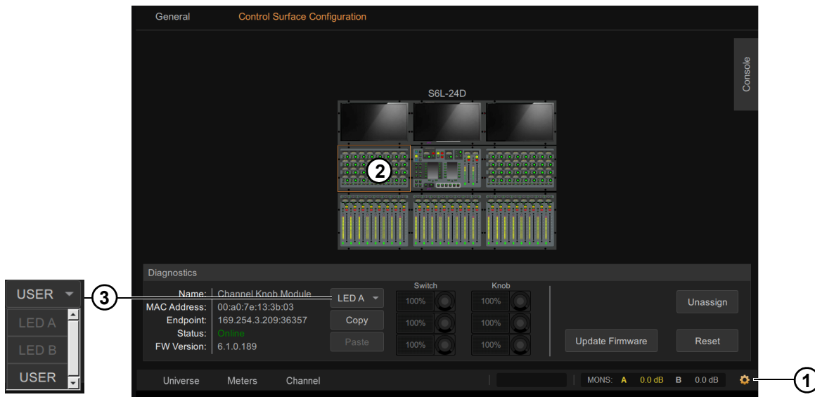
Control Surface Configuration view (MTS shown)
