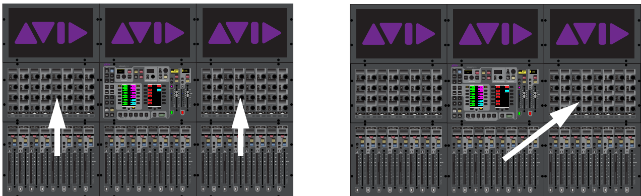
Selecting a channel below a CKM (left) and below the MLM (right) on an S6L-24D
