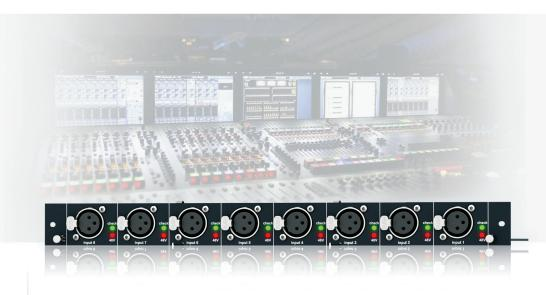
DL441 is a modular 8 channel analogue mic/line input and line level output card for MIDAS PRO Series control centres and modular I/O boxes, and features award-winning MIDAS microphone preamplifiers with switchable +48 V phantom power and servo-balanced electronic outputs with high current drive capability for long cable runs. Premium low latency 24 bit 96 kHz ADC and DAC converters
