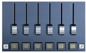
Below each fader you will find a screen button, you can use the left/right arrow to move this screen list. Each fader will transition the screen which is written on the button.
