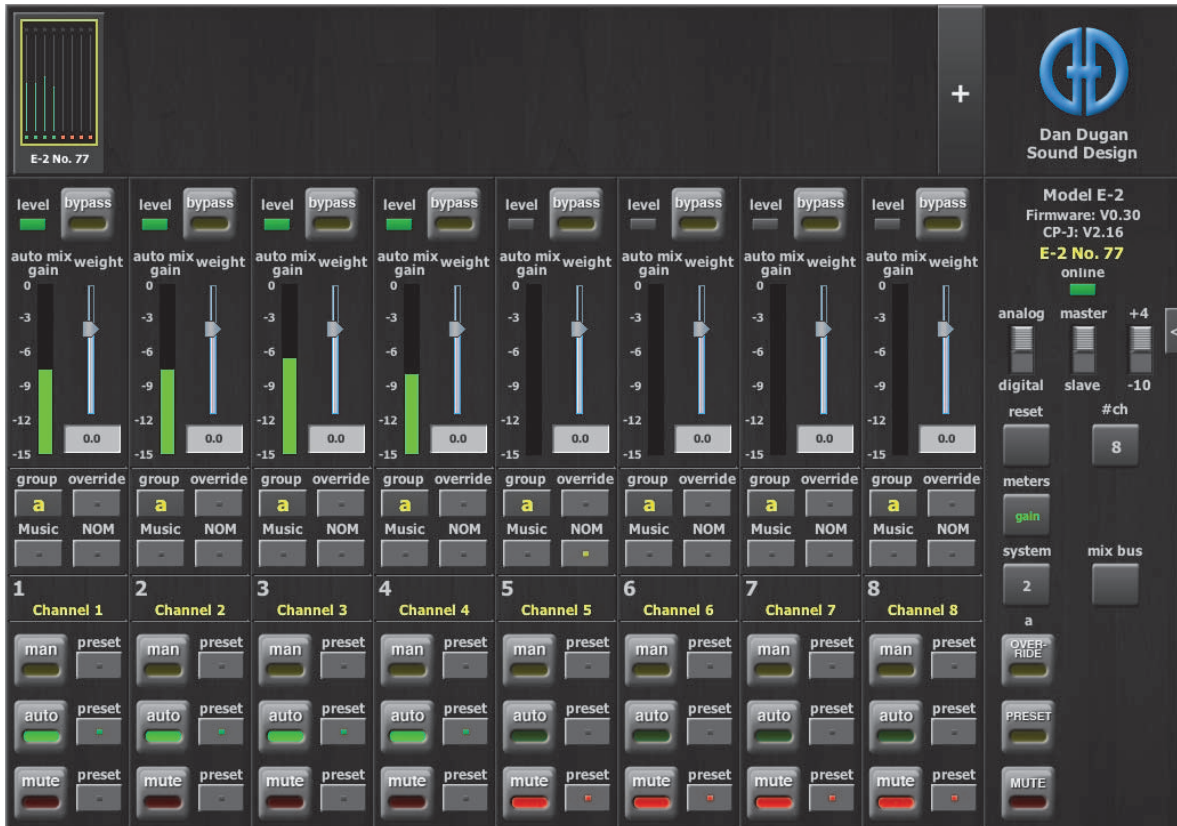
Figure 5-1 Dugan Control Panel
