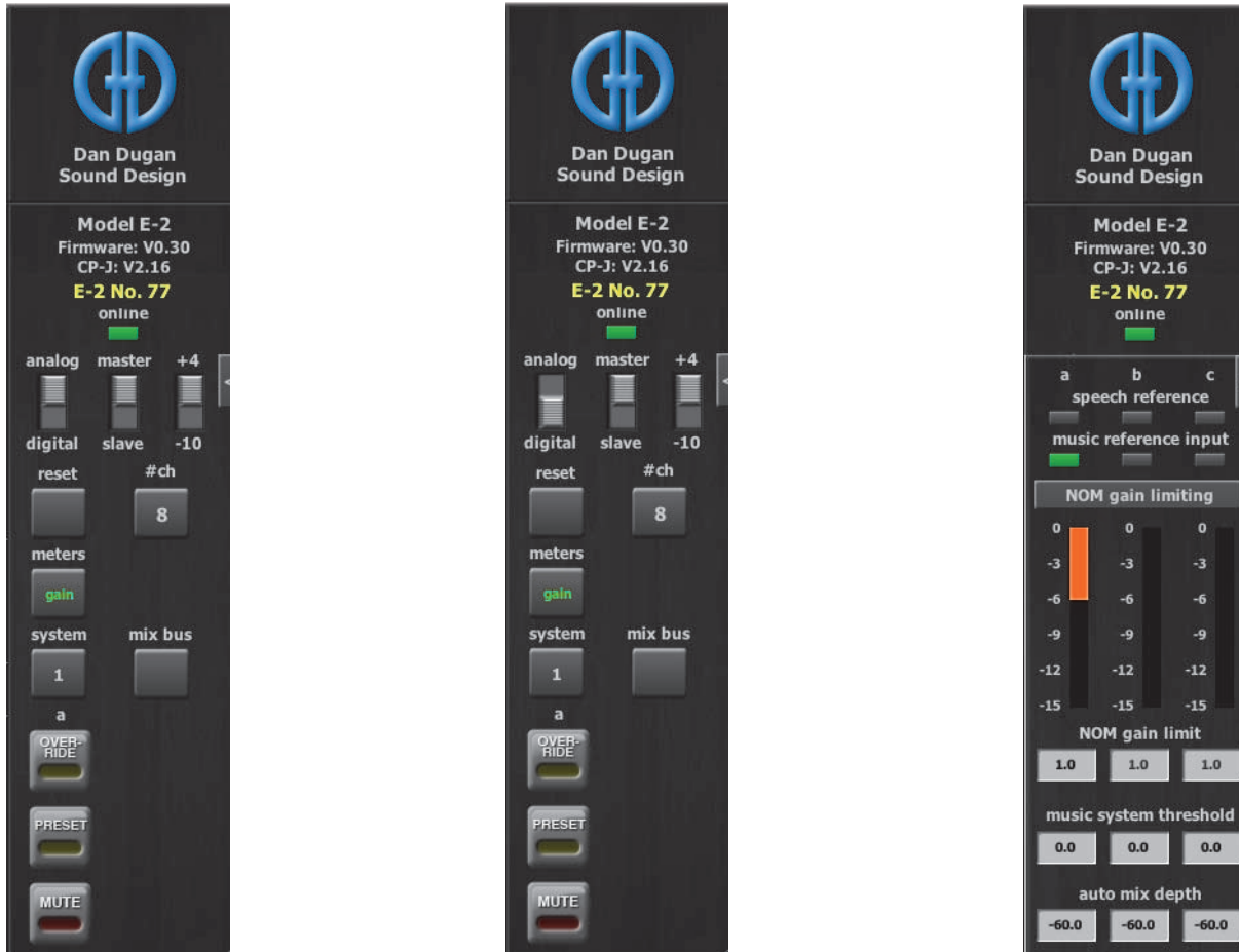
Figure 5-11 Master Pane: Analog settings (left), Digital settings (center), Music System controls (right)
