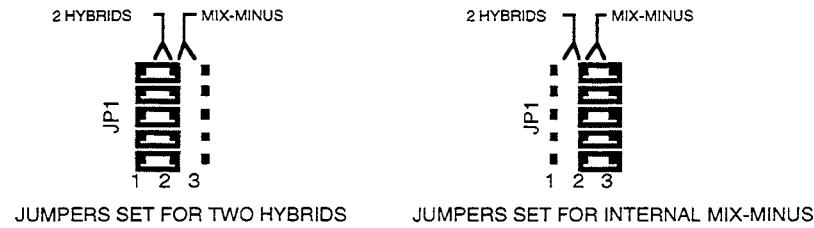
JP1 on rear panel connector board selects between two external mix-minuses or one external mix-minus cross-fed to both hybrids.
