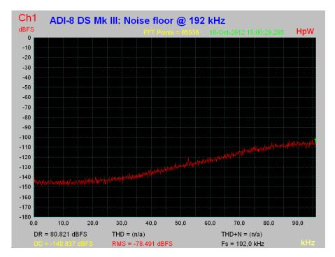
As can be seen in the above picture, the noise floor stays at a remarkably low level even outside the hearing range. At sample rates of up to 96 kHz the noise shaping happens completely outside of the transmission range.
