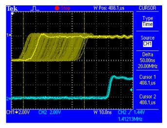
The cleaned and jitter-freed signal can be used as reference clock for any application, without any problem. The signal processed by SteadyClock is of course not only used internally, but also available at the ADI-8 DS' word clock output. It is also used to clock the digital outputs ADAT and AES/EBU.
