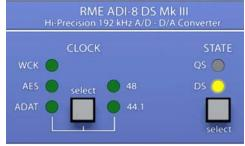
Using AES as clock source the STATE key is disabled, as the sample rate is clearly given by the input signal. ADAT misses such information, therefore when ADAT is clock source the STATE has to be set manually.
