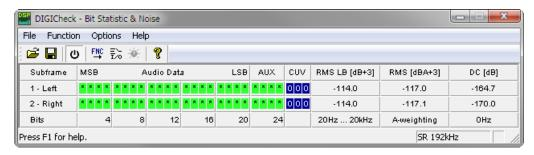
The reason for this behaviour is the noise shaping technology of the analog to digital converters. They move all noise and distortion to the in-audible higher frequency range, above 30 kHz. Therefore the noise is slightly increased in the ultrasound area. High-frequent noise has a high energy. Add the quadrupled bandwidth, and a wideband measurement will show a significant drop in SNR, while the human ear will notice absolutely no change in the audible noise floor.
