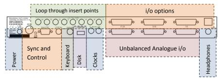
The lower 3 D-type connectors are the main Unbalanced Analogue i/o connectors on the BBP1U, BBP1A and BBP1D. The cable looms conform to the TASCAM standard for analogue i/o.
