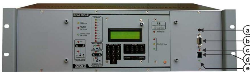
**a -** Switch fugitif allowing display serial number and carry out fade test of VCA
