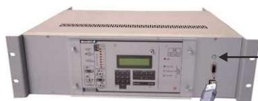
Fugitive switch to display serial number, and to test VCA fading..
