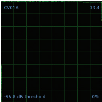
CD PLAYER INTO PHONO INPUT - The SL3 is set to receive a phono level input. Switch to the correct setting on the SL3.
