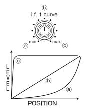
The curve characteristic changes from  $\textcircled{a} \rightarrow \textcircled{b} \rightarrow \textcircled{c}$  when the volume knob is turned clockwise.
