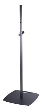
Attractive lighting stand. Thanks to the heavy, flat steel plate the stand is well suited for use in small areas. The proven safety bolt with locking screw provides for comfortable and safe height adjustment. The stand?s maximum extension height is 2.400 mm and maximum weight is 18 kg. The integrated M10 threaded bushing provides for the attachment of crossbars.
