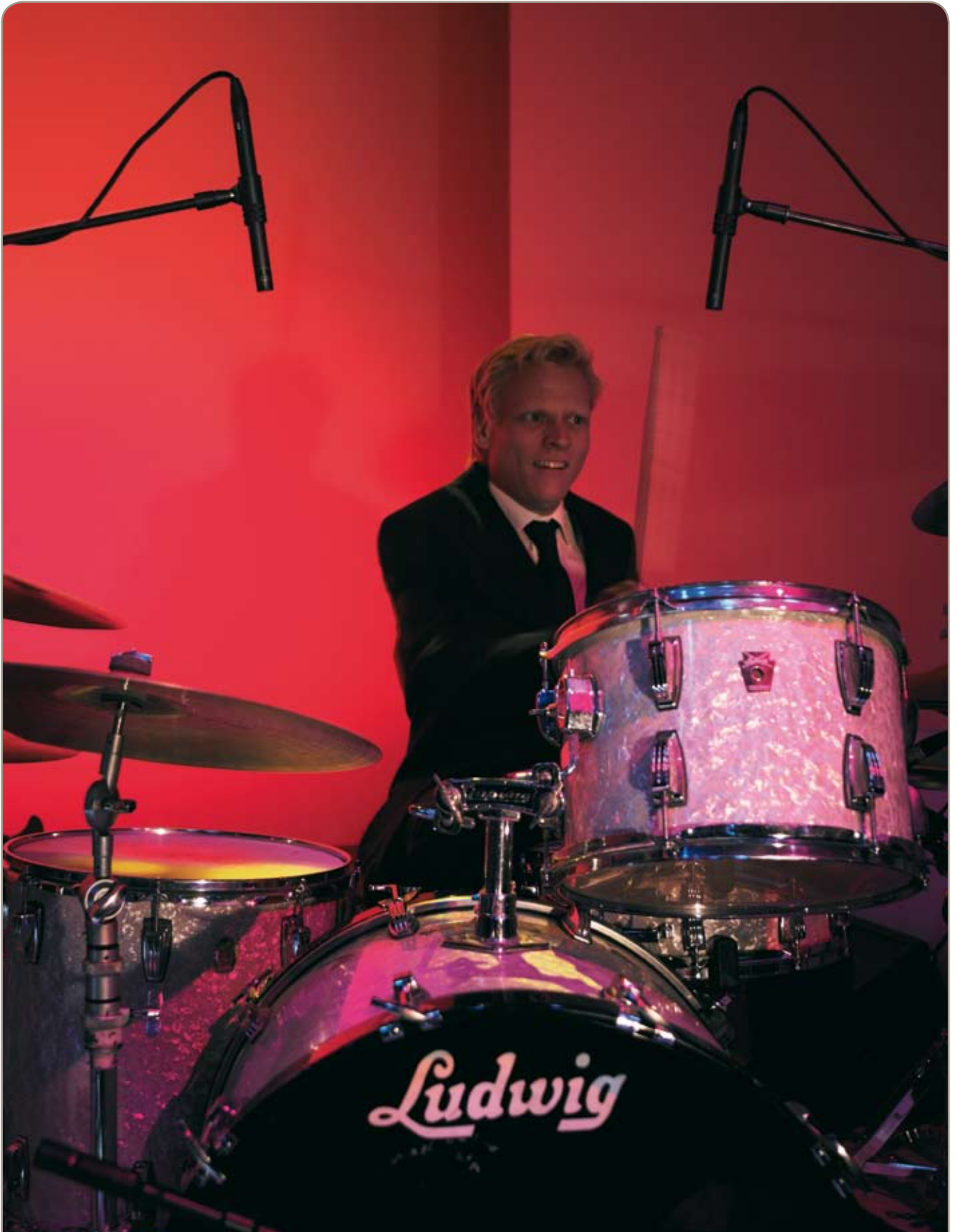
A pair of 4011-TL microphones is a serious overhead miking solution to capture the sound, width and dynamics of the drum kit as it is.
