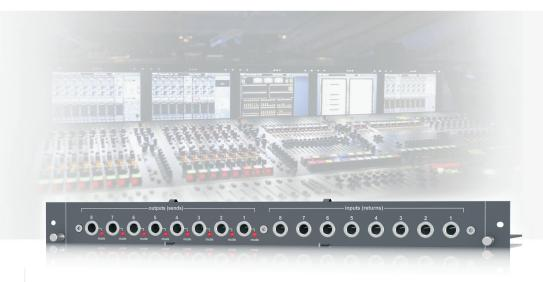
DL443 is a modular 8 analogue line level input and output card for MIDAS PRO Series control centres and modular I/O boxes Premium low latency 24 bit 96 kHz ADC and DAC converters are used to minimise distortion and noise artefacts, and DL443 features balanced inputs and outputs on ¼" TRS connectors high common mode input noise rejection and high output current drive
