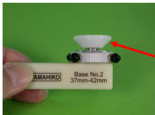
And **Contact tip** is installed.
