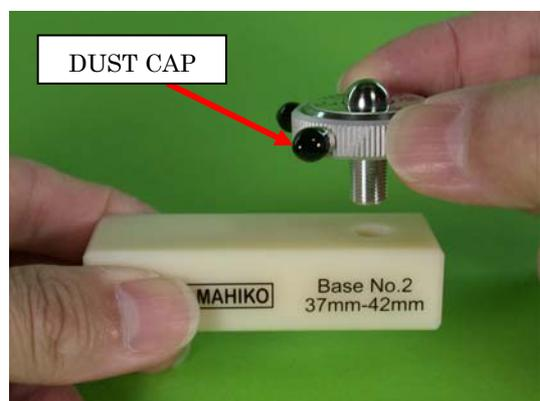
Then put **the sensor** into the selected **base**, screwing it into the hole of the **base** until the bottom part of **the sensor** touches on the surface of **the base**.
