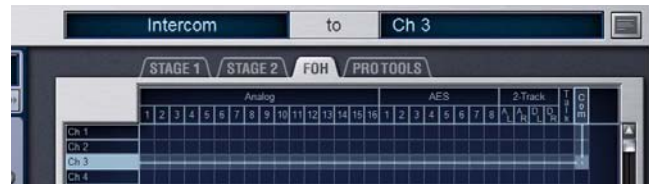
Routing Intercom input in the Patchbay
