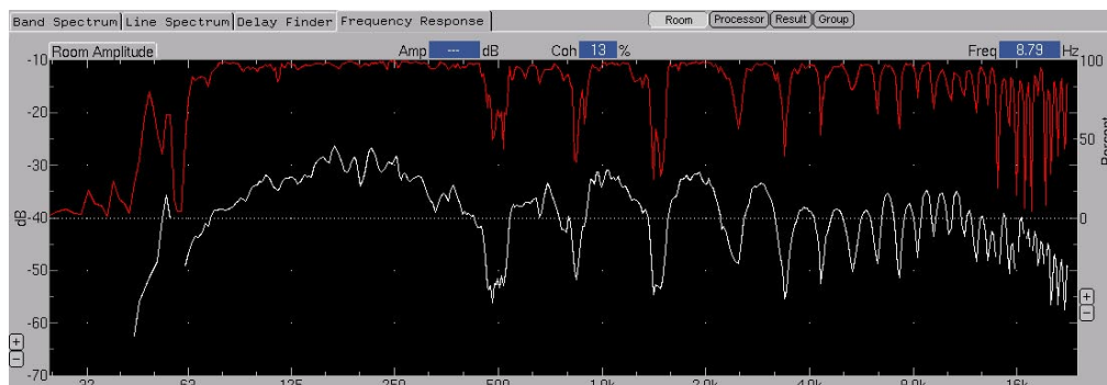
Figure 7.27. Frequency Response trace showing comb filtering
