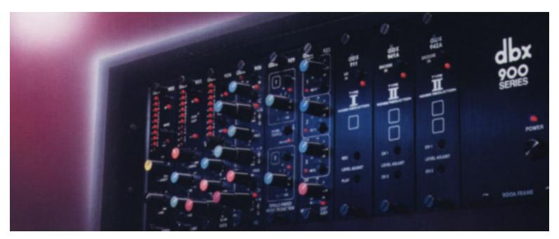
The F900A is the foundation for creating a customized "audio toolbox." It holds up to 9 dbx 900 series modules in a 3U rack space. Standard barrier strips provide access to all input and output connections. To ensure reliability and consistent performance under the most demanding conditions, all internal connections to modules are made via double-sided, gold, bifurcated contacts.
