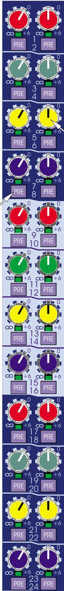
The aux PRE switches only operate when in one of the AUX bus modes; they change the signals sent to the group busses from post fader to pre fader.
