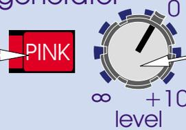
The generator **LEVEL** control gives continuous adjustment of the signal generator peak output signals from +10dBu to off.
