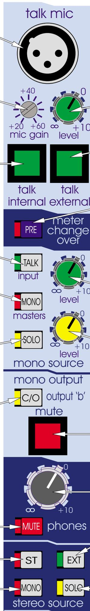
The talk LEVEL gives continuous adjustment of the post limiter signals from +10dB to off.
