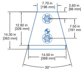
The UPA-1P loudspeaker provides high power output, low distortion, and consistent polar response in a compact, vented two-way enclosure. The loudspeaker features a 12-inch cone low-frequency driver and a 3-inch diaphragm compression driver coupled with a 100° horizontal by 40° vertical constant-Q horn. The versatile UPA-1P has a variety of sound reinforcement applications including as a main front-of-house loudspeaker in small- to mid-sized venues and as a fill loudspeaker in larger systems.
